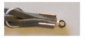
• Squeeze the clamp closed using needle nose pliers
